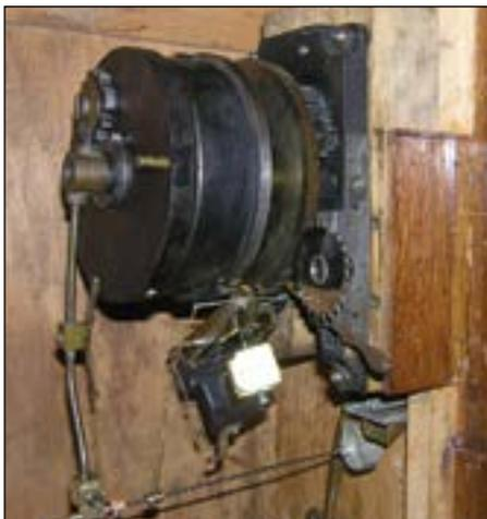
Figure 20: With the bedplate removed, shown is an angled front view of the Criterion spring motor and coin mechanism from the machine in the Klish collection.
