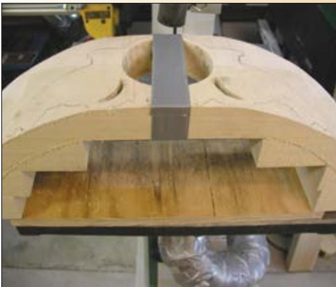
The front profile is now cut on the band saw and the cutouts are drilled out and shaped with a chisel.
