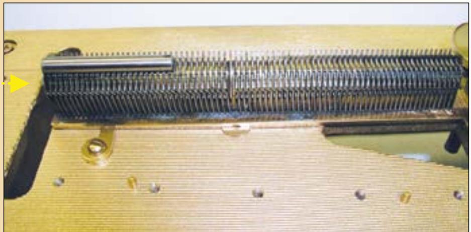
The dampers should all be uniform in appearance and positioned with tension against the star wheels. If this step is done carefully the dampers will most likely not need much attention later when the comb is installed.
