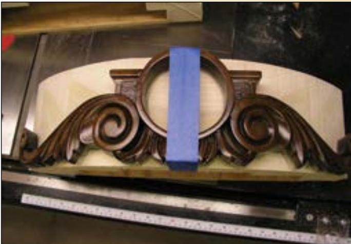
The original crest is now laid over the cut wood to trace the front profile and cutouts.
