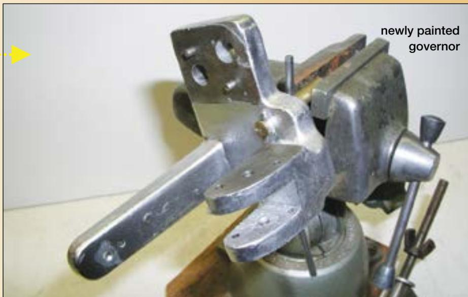
Now that all of the governor parts have been cleaned and polished it is time to reassemble the governor. First start with the side plates and the two gears that go between them and assemble these onto the casting or metal part that separates them.
