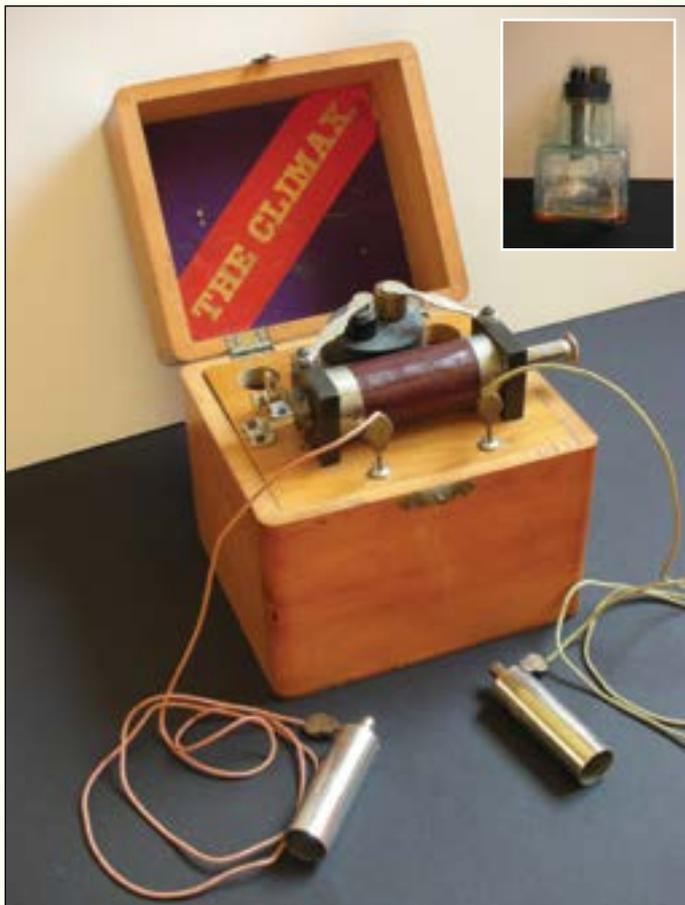
The smallest example of an Otto shock machine in my collection is "THE CLIMAX." This view shows the box open with grippers plugged in and ready for action. The glass jar battery (inset) is shown here with its elements and also the name F. G. Otto & Sons, Jersey City cast into the front of the glass.
