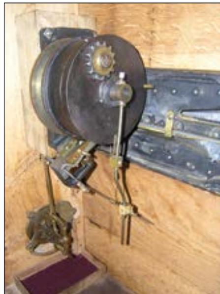
Figure 21: Another angled view of the Klish mechanism, but this one is taken from the back side. This shows the heavy brass arm connected to the coin slide that released the ball dispenser, the money shovel and the cast iron spring barrel.
