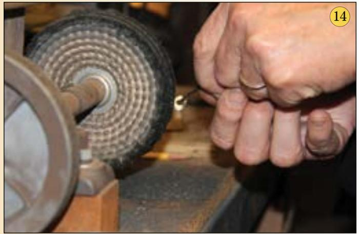
In addition the washers used under the comb screws can be polished with a wire wheel or buffer by placing the washer on a nail so that it is free to rotate against the nail head.
