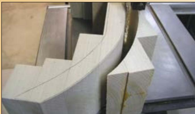
A pattern is first made of the front to back profile of the crests as shown at right. The glued wood is then cut on one side using a pattern from the originals.
