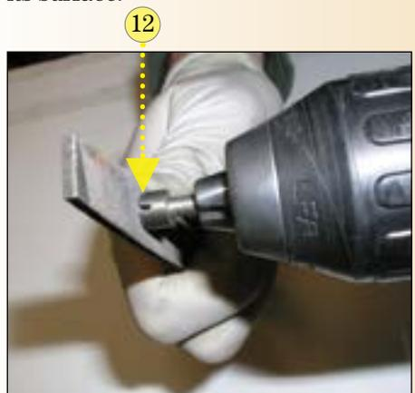
The screw head can be cleaned and wire brushed and/or polished using the drill motor while turning. The degree of polish will vary depending on the polish on the rest of the music box. Some music boxes have a high degree of polish on all of the parts and some have a satin appearance. Wire brushing will get the rust off and give a satin appearance, if a higher degree of polish is desired the screw can be buffed as well.
