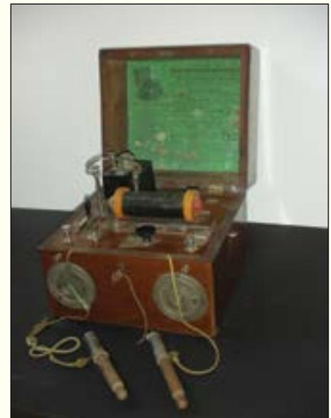
Dr. Drescher’s “THE IMPROVED 1 CELL ELECTRO-MAGNETIC No. 3” has two dials on the front of the box to let out the electrical cable or reel it back into the case.
