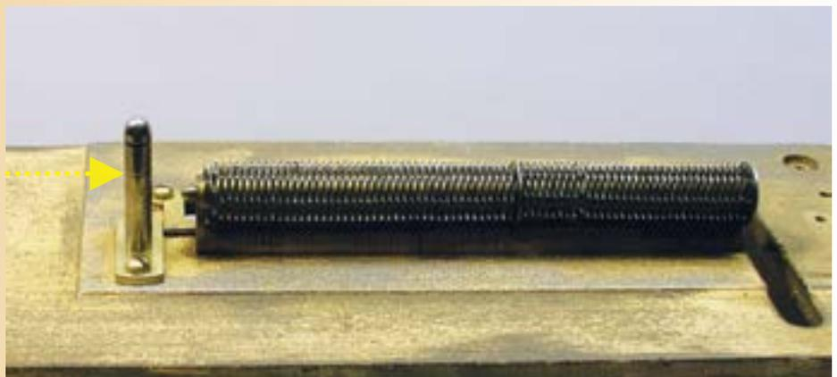
Removing the center post is not usually necessary but if it must be removed the following is a useful technique. Follow these instructions closely so that the center post can be put back in exactly the same position as it was. Clamp metal bars to hold the bracket position side to side as well as up and down as shown. This way the bracket can be perfectly repositioned during reassembly.
