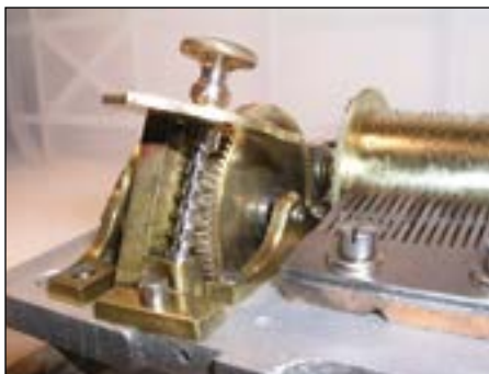
Wider view of the replacement worm gear and mating spur gear.
