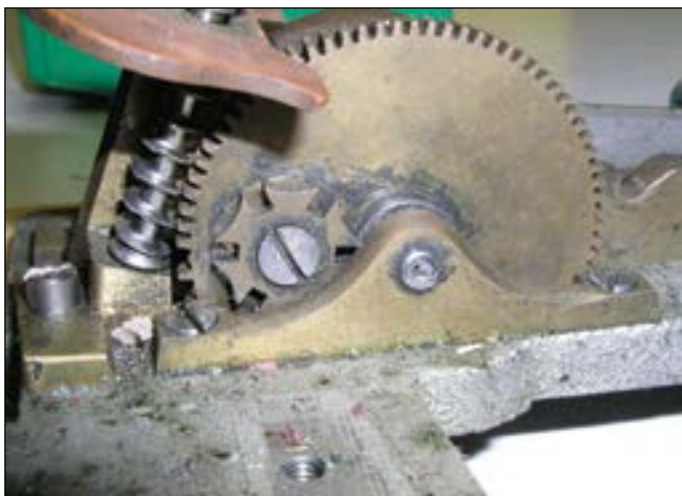
A close up of the broken gear teeth and damaged worm gear that would both need to be replaced.
