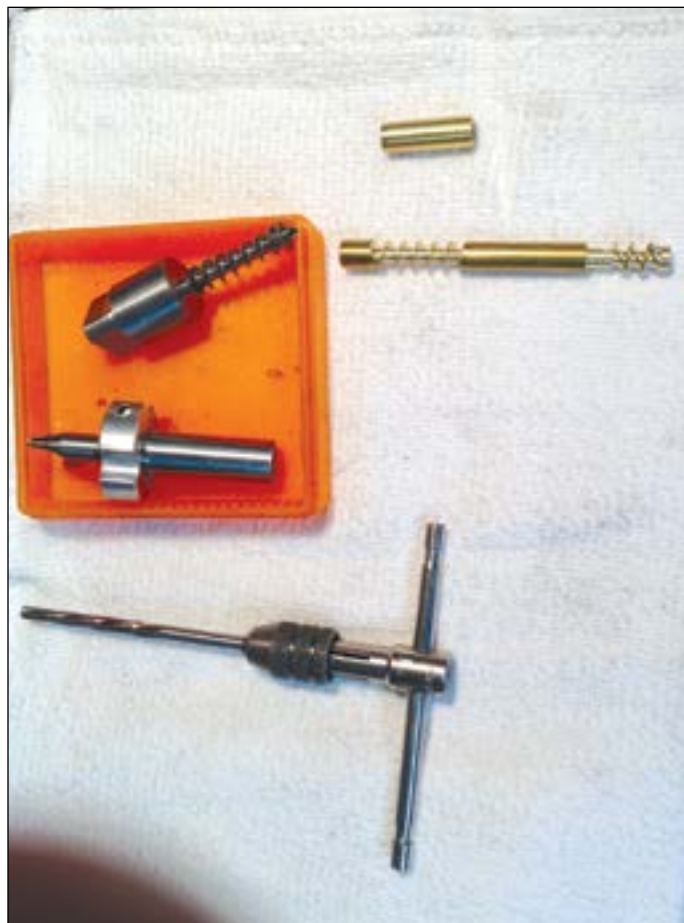
View of trial worm gears made to check set up accuracy
