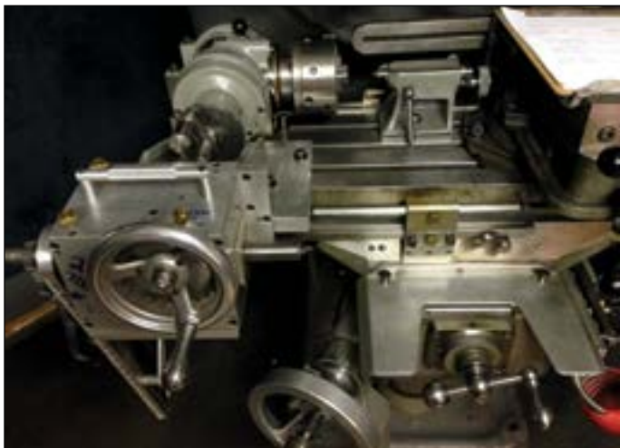
Worm gear machining set up.
