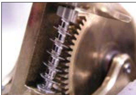
Close up of new worm gear and mating spur gear installed.
