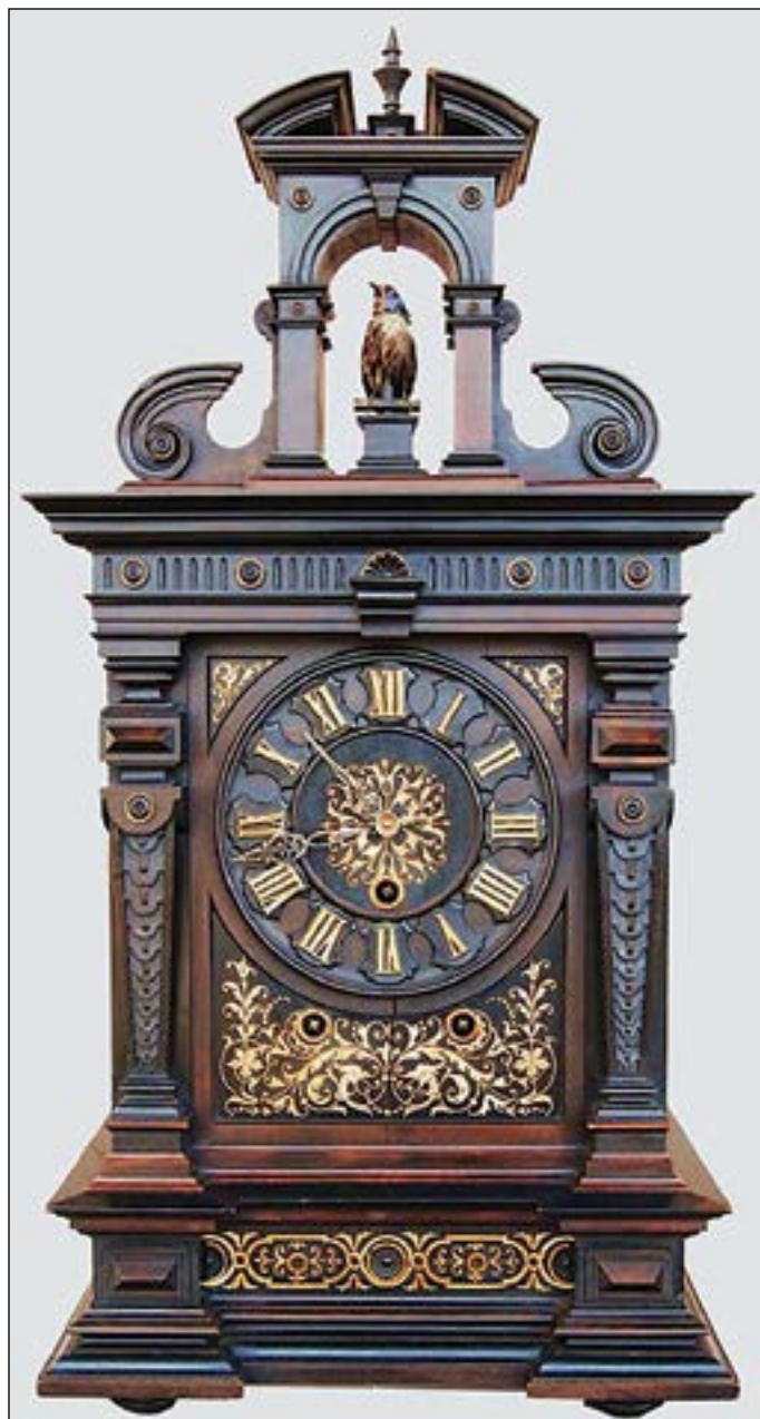
A shelf singing bird clock made by Emilian Wehrle & Co., circa 1875. This example is equipped with a solid brass plate, three-train movement that runs for eight days. After striking the hour on a large gong, the full-feathered bird located in the upper arch of the clock comes to life. The bird has automation to the beak, head, and tail, which all move in perfect sequence to the bird's song. The ebonized case has extensive accents in gold. The backboard is inscribed by hand and dated in German. The inscription states that this clock was made by Emilian Wehrle in 1875 and gives the information of its first purchaser, who purchased the clock in 1876.
