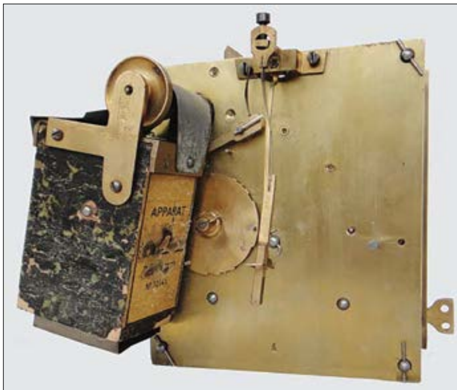
Located on the back of the rooster clock movement is a small wooden “sound box.” The box is attached to the movement by a metal arbor, allowing it to pivot on its axis. On the top of this small wooden box is a serrated wheel. This wheel rides on a thin metal reed that extends across the top of the sound box. When the serrated wheel is spun, it vibrates the reed, causing the sound to echo through the sound box. On the back of the movement is a small, precisely cut, cam wheel. The cam wheel controls the amount of pressure applied to the serrated wheel, thus controlling the pitch of the call. On the hour (or on demand), the movement activates the cam wheel. The rooster's crow is reproduced by the varying speed at which the serrated wheel is spun. The cam wheel also controls the automated rooster located at the top of the clock. As the movement produces the call, the rooster leans forward and opens its beak before tipping back and letting out his crow as the beak slowly closes. The rooster crows three times on the hour.
