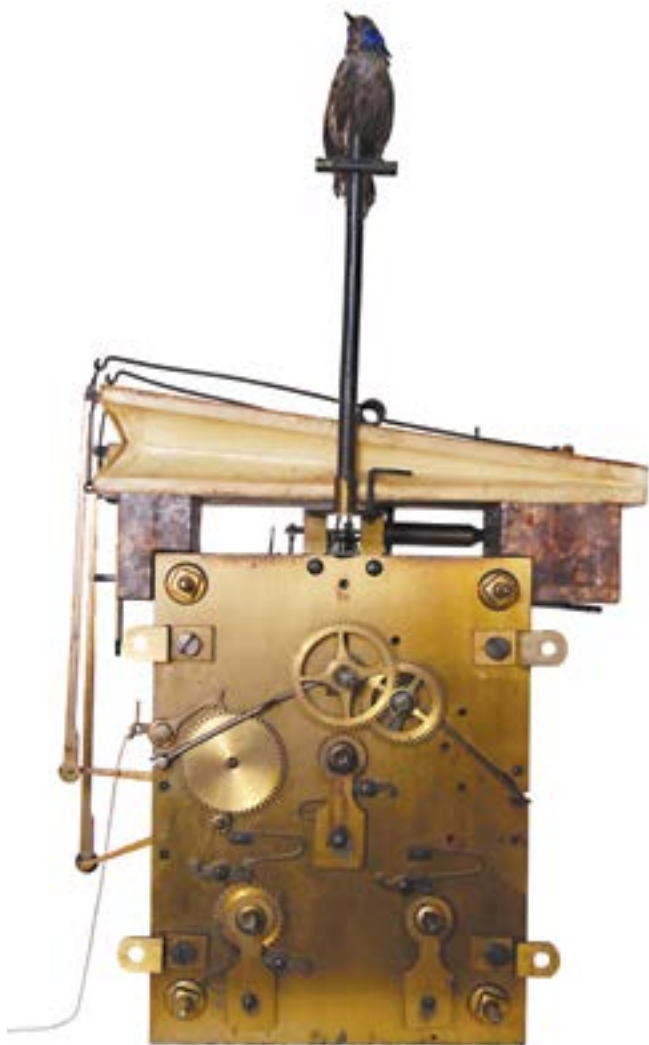
The singing bird movement removed from the case. Instead of a large pinned wood musical wheel found on the flute and trumpeter clocks, the singing bird clock has a large cam wheel machined from brass.
