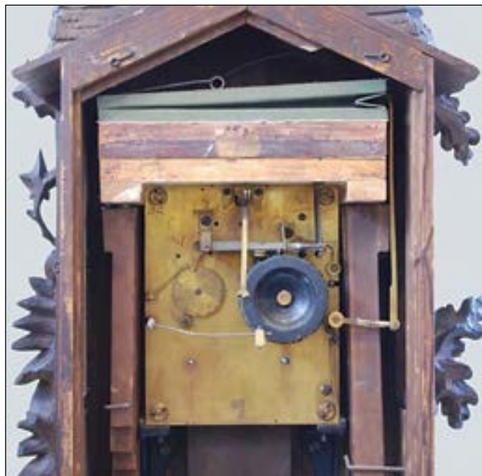
This flute clock movement is nearly identical in every way to the trumpeter movement described in Part 1 of this article. By replacing the metal horns and reeds with wood pipes, the clock produced a much more mellow and softer sound. Today some collectors prefer the sound of the flute, while others favor the louder trumpeters. The firm produced more clocks equipped with the trumpeter, making the Wehrle flute clocks more difficult to locate today.
