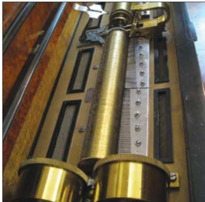
This is an inline duplex cylinder musical box, which is rarer than a parallel duplex box.
