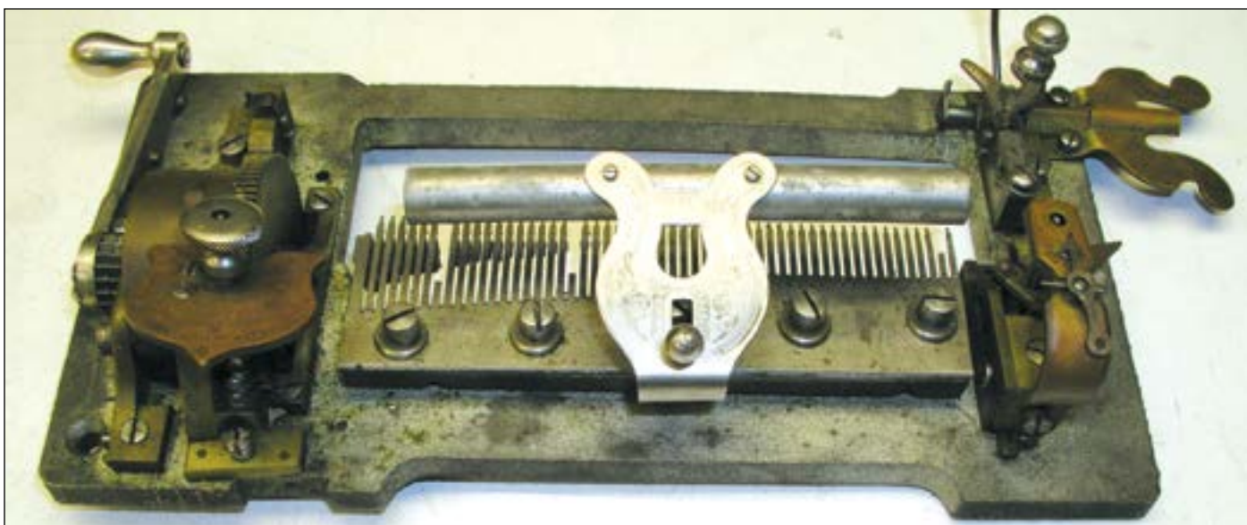
The comb had several broken teeth and the bedplate plus associated parts were grimy with age.
