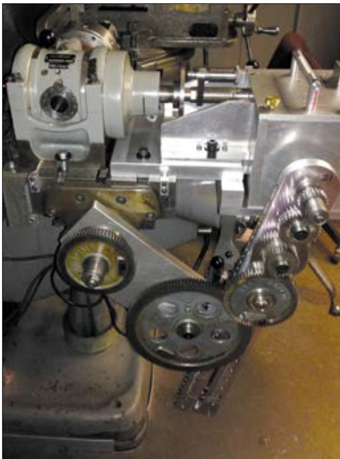
Worm gear machining set up showing gear changes.
