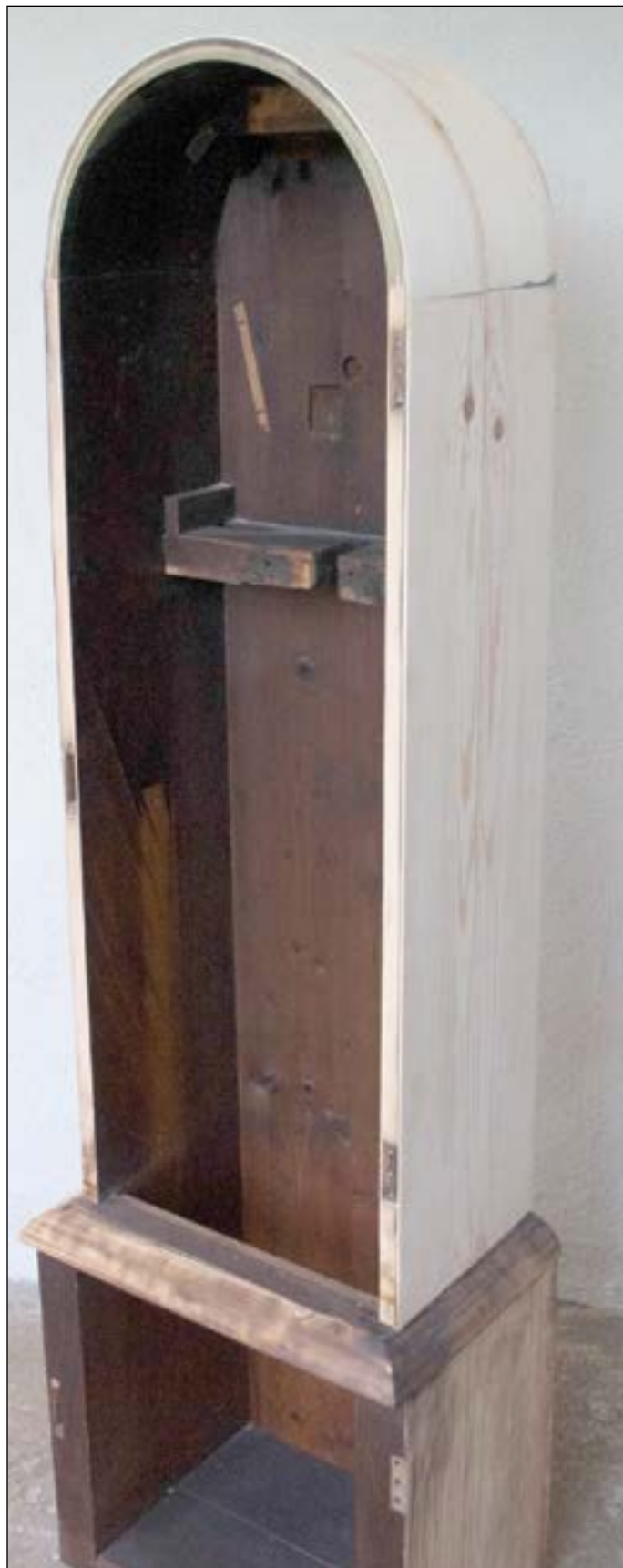
Another view of the case showing the new pine substrate prior to oak veneer being applied.
