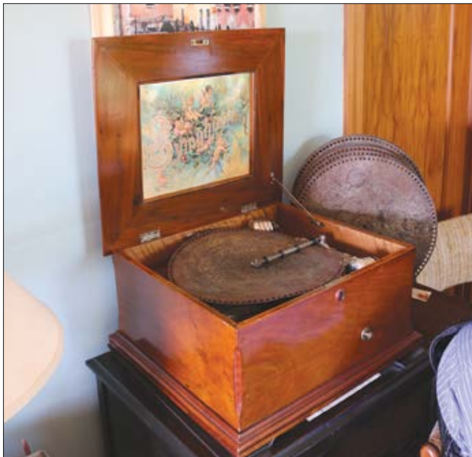
Symphonium Style 121GI 14 \frac{3}{4} inch disc box with 10 saucer bells.
