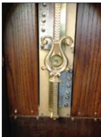
The restored baseplate and coin slot.
