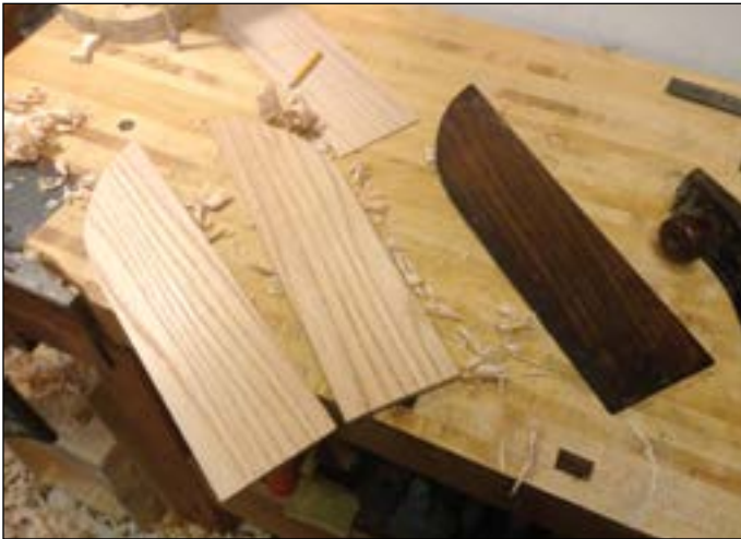
New matching oak fascia were bandsaw cut and planed. These go inside the case on either side of the bedplate.
