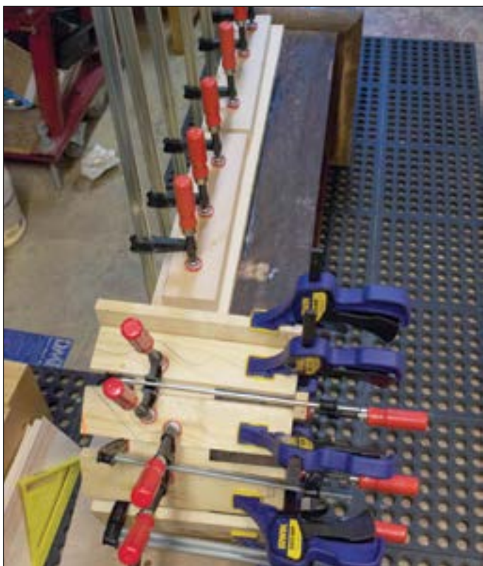
A new pine wood substrate being applied using epoxy and wood cauls.
