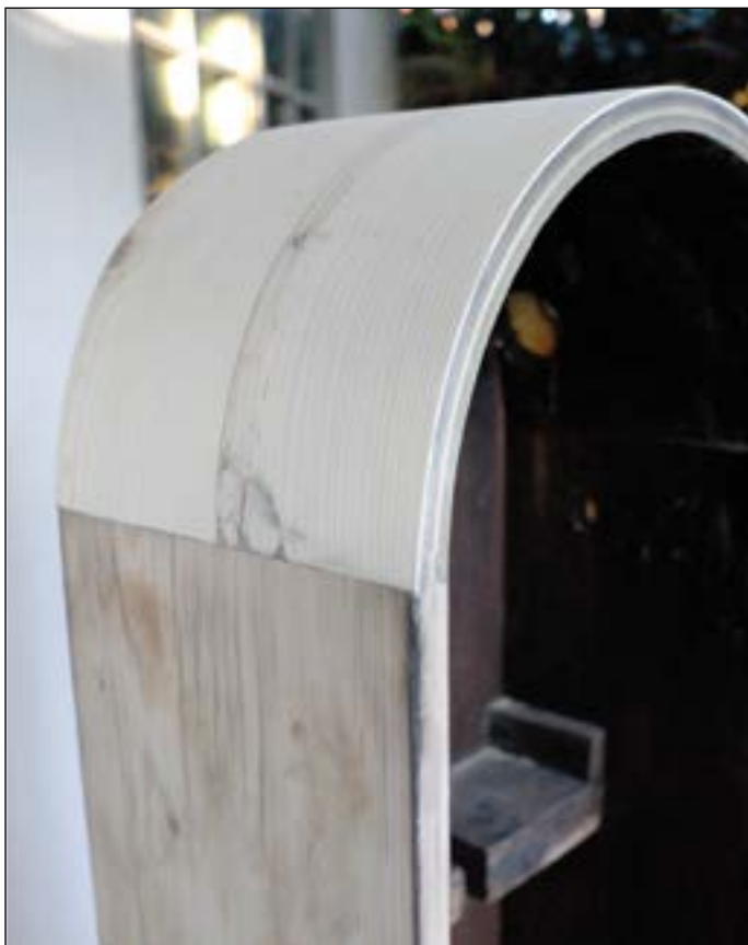
One view of the curved top of the case, prior to veneering.
