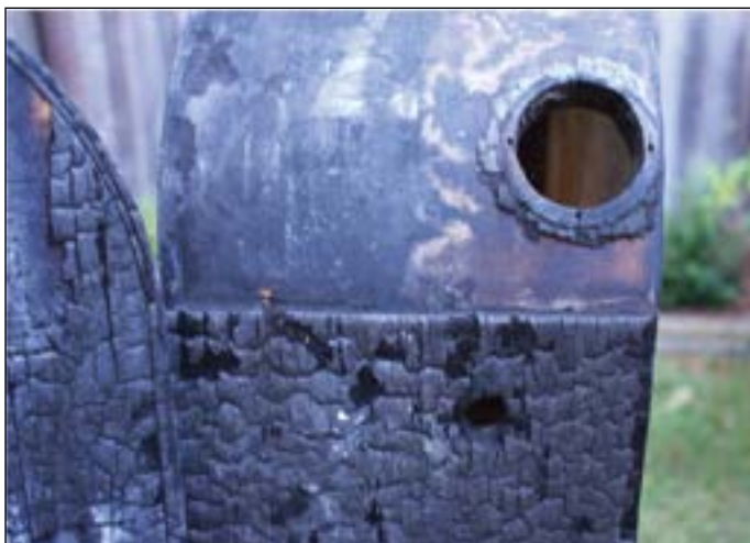
The burned area around the coin slot.
