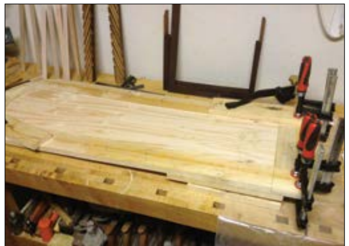
The front door, being glued to fit the case.
