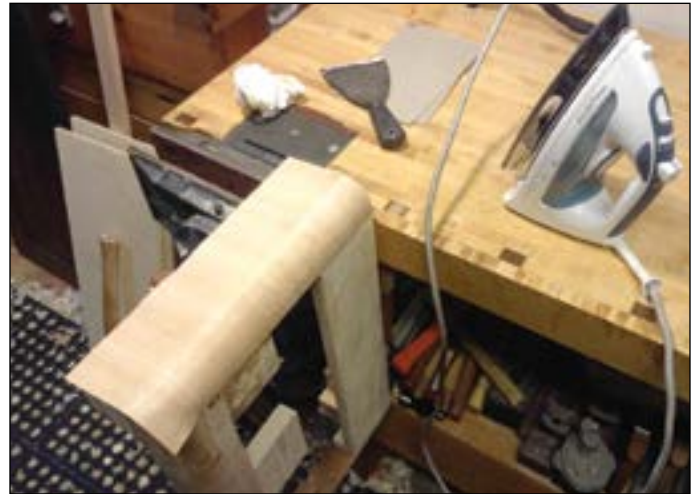
In this picture you can see where the veneer was steam bent over curves.
