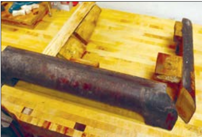
The base as received. The hide glue and supporting blocks that held it together have separated.
