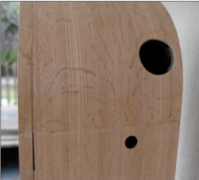
In this side view, you can see the flow of the wood grain over two pieces of veneer.
