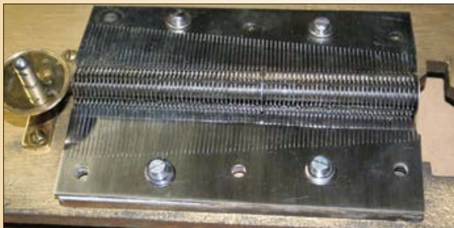
Figure 35: The new comb installed on the bedplate and ready for action.
