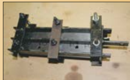
Figure 13: Third blank clamped into the heat treat fixture.
