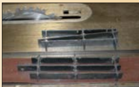
Figure 6: The two-part heat treat fixture.
