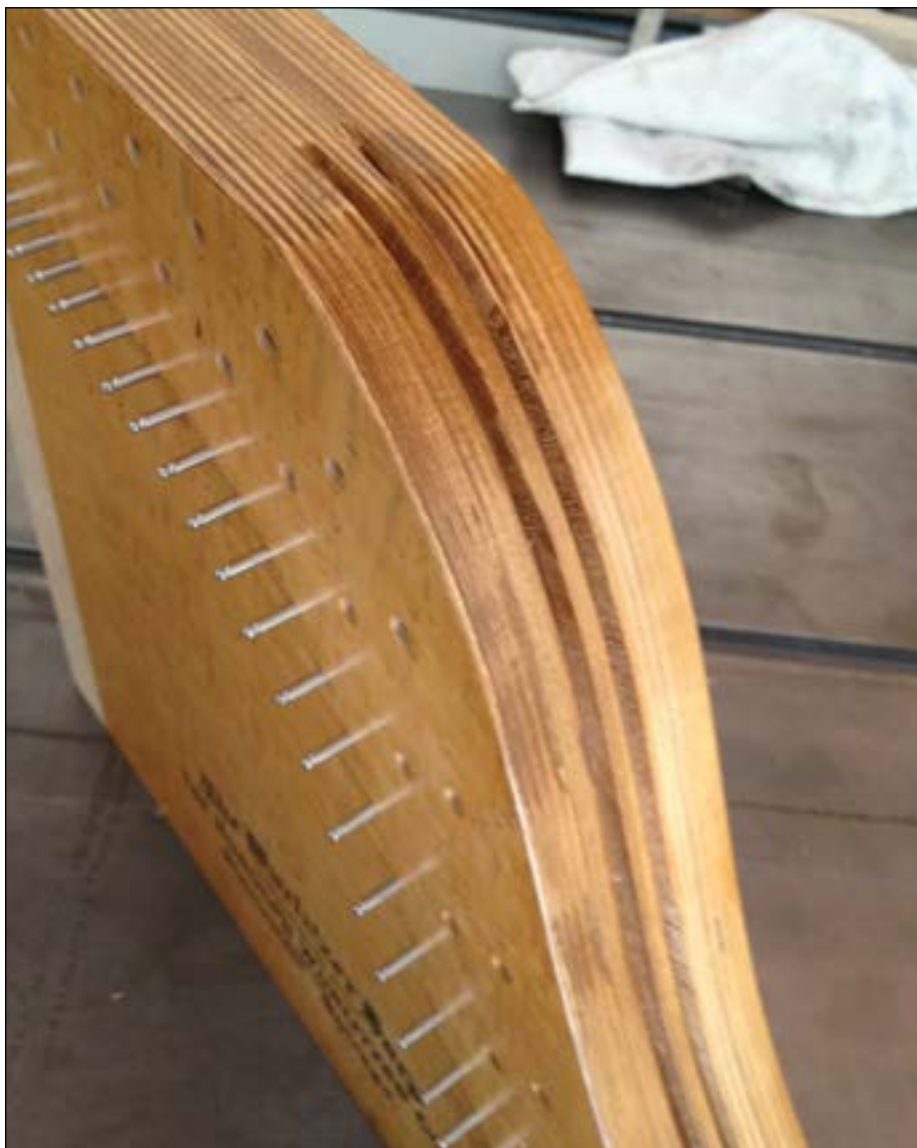
The new pin block, double stained to match the original color.
