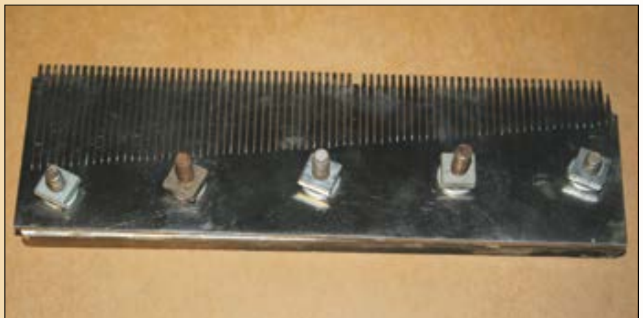
Figure 28: The remaining bolts and lock washers are installed.
