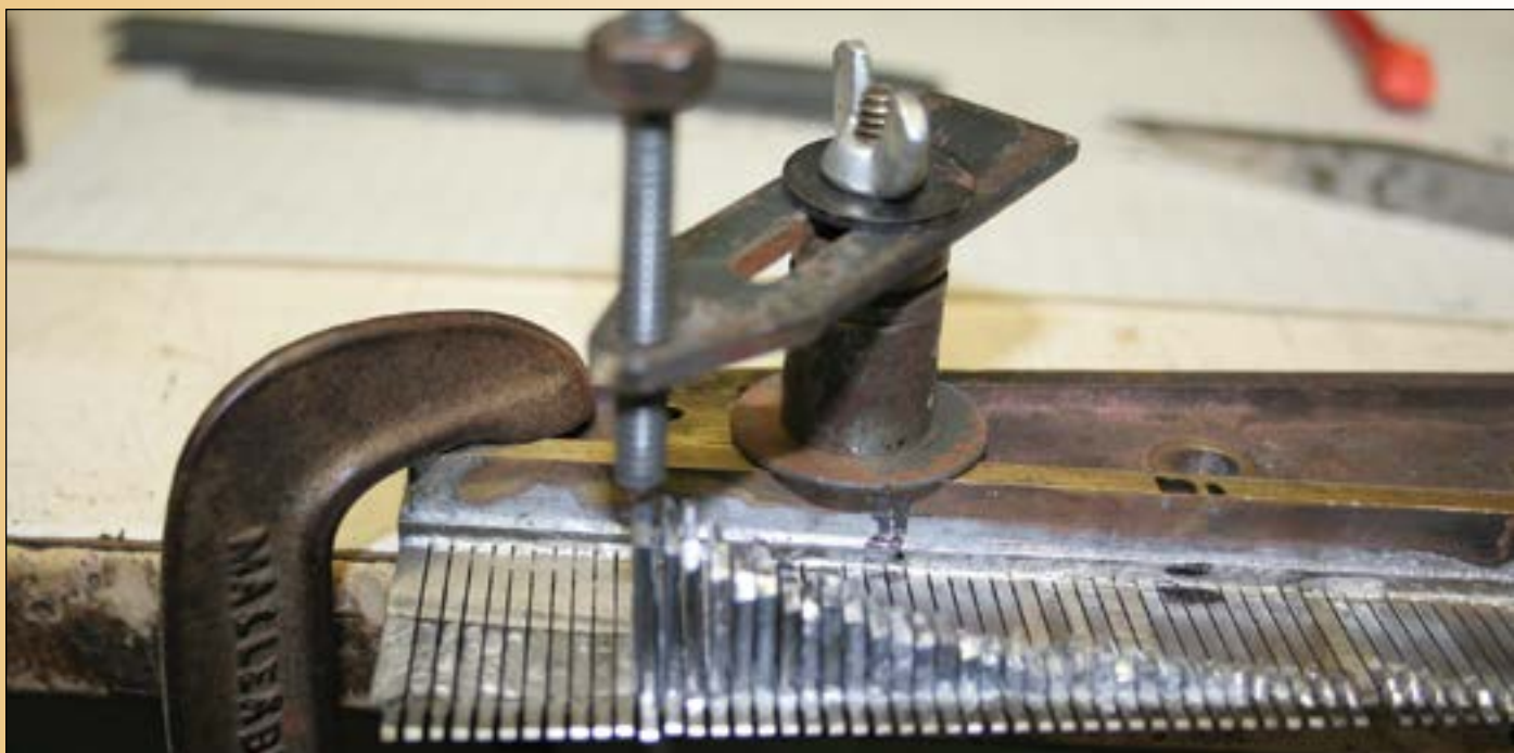
Figure 33: The comb is tuned except for the lower area with the bass notes.
