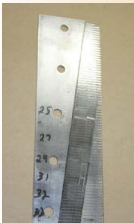
Figure 22: All the teeth ground to the correct thickness.
