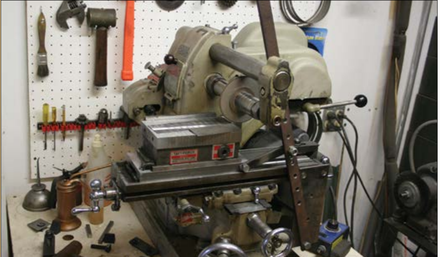
Figure 20: The setup for grinding the underside of the teeth on the new comb.
