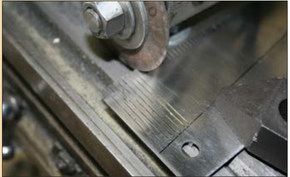
Figure 18: Cutting out each tooth to the marked layout line.
