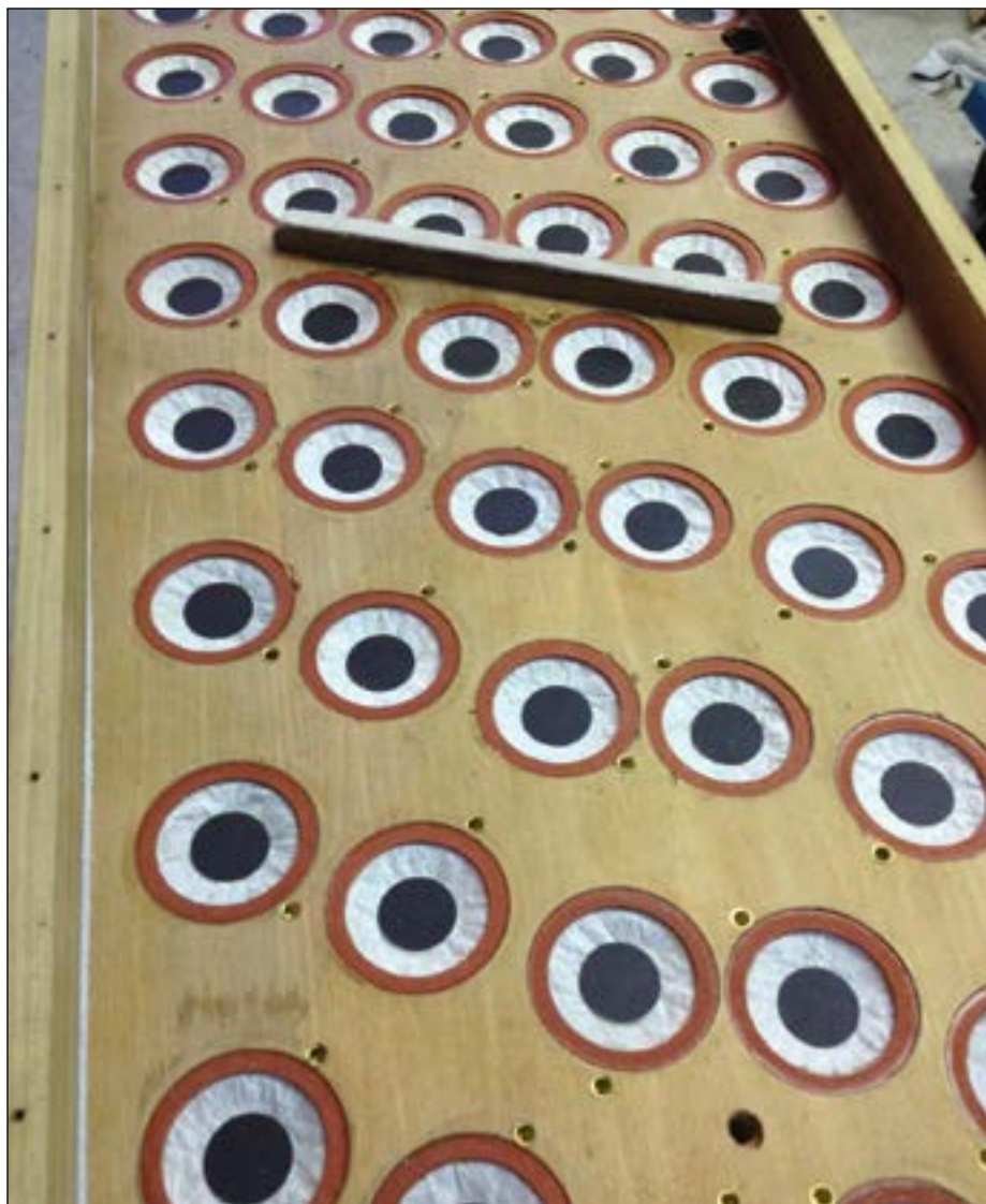
The rebuilt valve chest.
