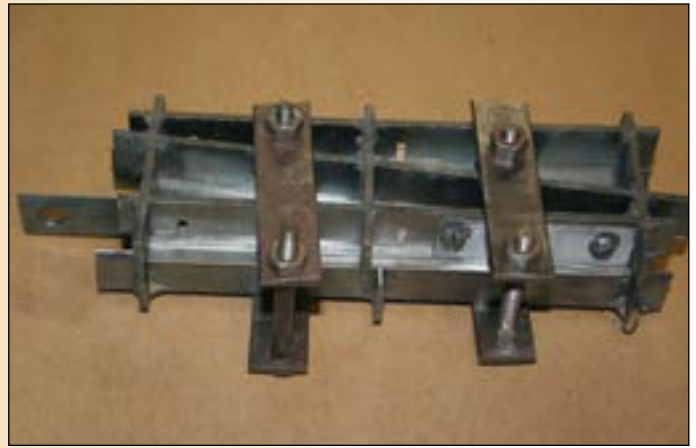
Figure 8: The heat treat fixtures clamped around the steel comb blank before placing it in the kiln.
