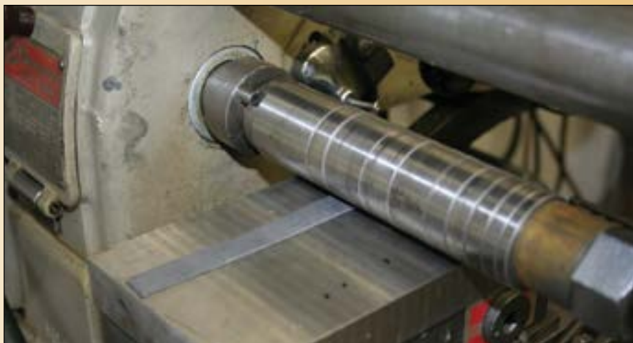
Figure 31: Rolling the lead that will be cut as needed for weights.
