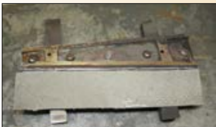
Figure 29: Asbestos cloth protects the teeth during soldering.
