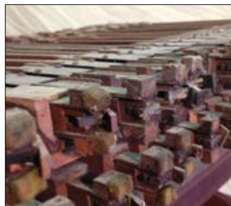
The original oak pluckers were worn and in need of restoration.
