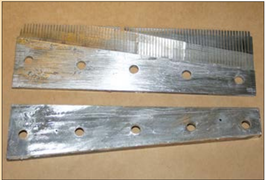
Figure 26: After removal of the brass plate from the old comb.
