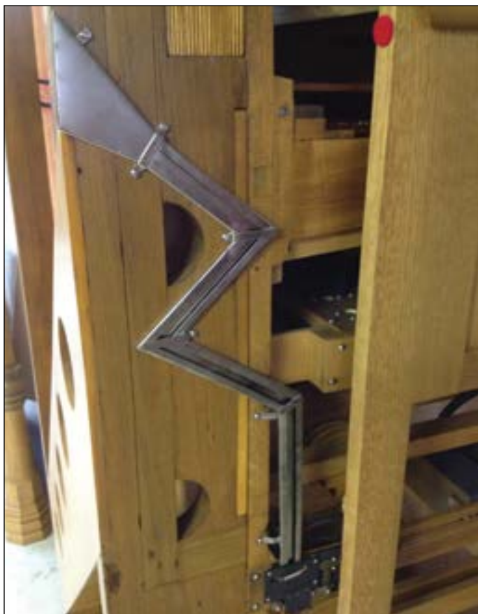
A new coin shoot made out of brass and nickel plated.
