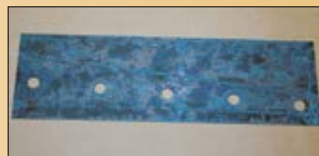
Figure 14: Third blank after heat treatment, showing coating of scale.
