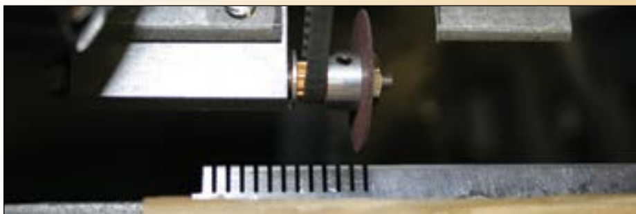
Figure 16: Grinding new tooth tips using the pitch from the old comb.
