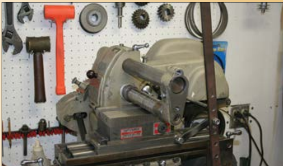
Figure 30: The setup for creating a length of lead at the proper thickness. Note that the long handle is still installed on the machine.
