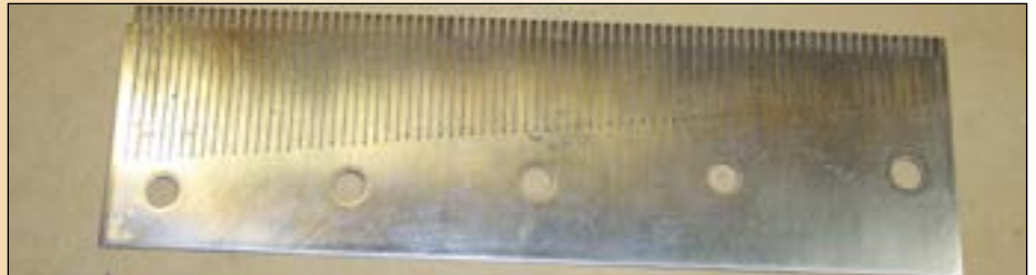
Figure 19: All the teeth cut to the proper length.
