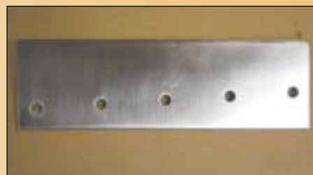
Figure 15: After polishing, a straight usable blank is ready to be milled.
