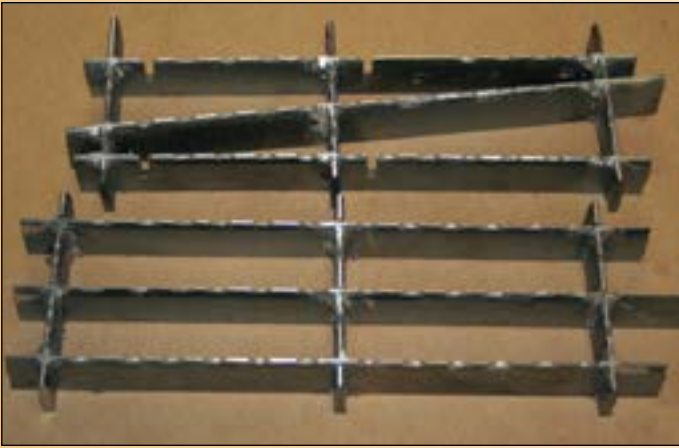
Figure 7: The slots in the heat treat fixtures minimize contact with the steel comb blank.
