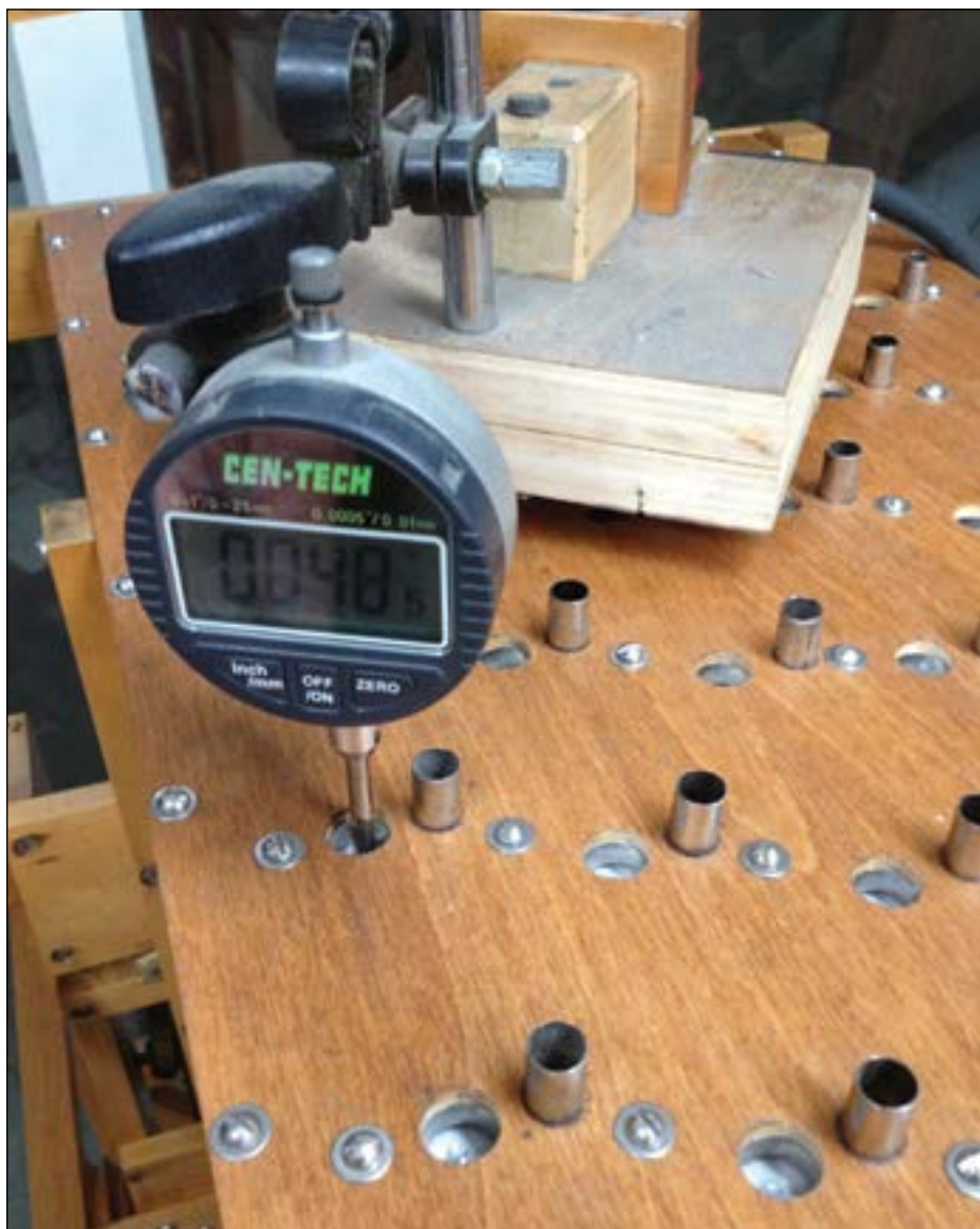
Measuring for optimal valve travel with a digital calibration unit.
