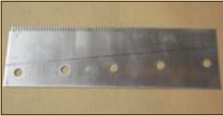
Figure 17: All tooth tips ground.
