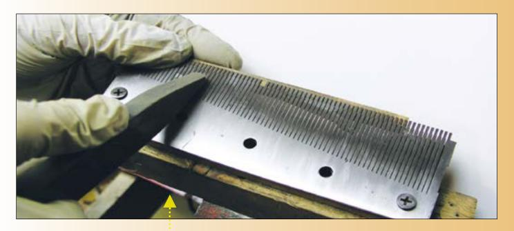
The comb is next degreased if necessary, and a Cratex abrasive bar is used to clean up surface grime and light rust from the comb without
