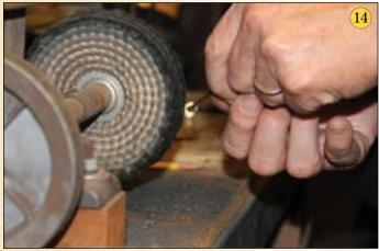
In addition the washers used under the comb screws can be polished with a wire wheel or buffer by placing the washer on a nail so that it is free to rotate against the nail head.
