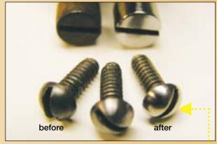
The screw head can be cleaned and wire brushed and/or polished using the drill motor while turning. The degree of polish will vary depending on the polish on the rest of the music box. Some music boxes have a high degree of polish on all of the parts and some have a satin appearance. Wire brushing will get the rust off and give a satin appearance, if a higher degree of polish is desired the screw can be buffed as well.
