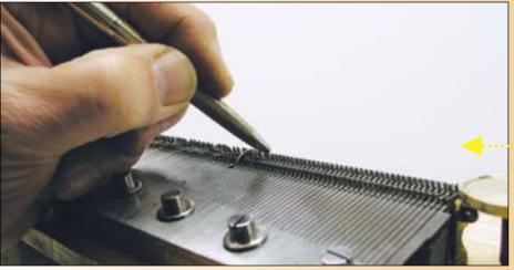
The Cratex abrasive is stroked across the comb in the direction of the teeth tips so as to not leave any cross scratches while the teeth tips are supported with a small piece of wood. After the comb is cleaned in this manner the comb is sprayed with lacquer or oiled to prevent corrosion.
