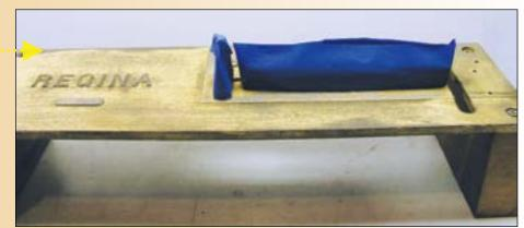
The bedplate is now painted gold and we are ready to align the star wheels with a dowel pin. This facilitates assessing how well the dampers are adjusted.
