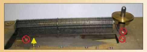
Clean out the dirt and dust from the dampers being very careful not to bend the dampers. Never loosen or move the star wheel gantry, damper rail, or center post as these were set at the factory and are very difficult to get back in the right place.
